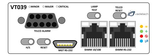
Figure 2: VT039 Front Panel View
