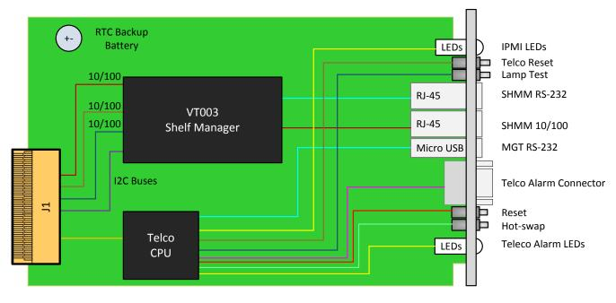
Figure 1: VT039 Block Diagram
